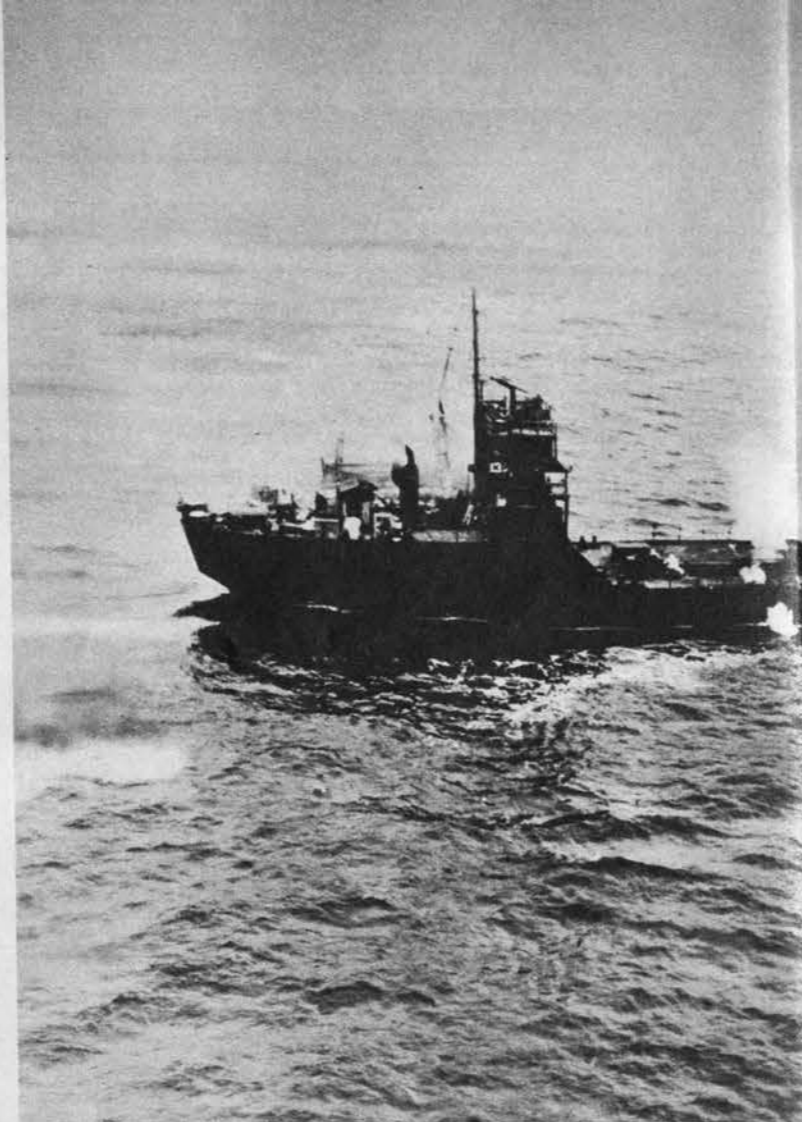
Low silhouette is afforded by Sugar Able Sugar. It has sharply raised forecastle bow, faceted stern found on most of important standard
